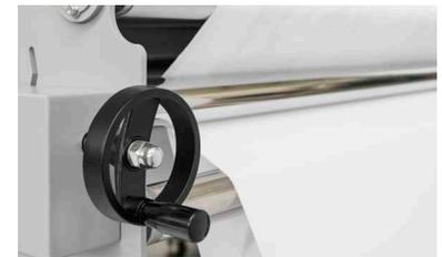
Fabric tensioning adjustment
